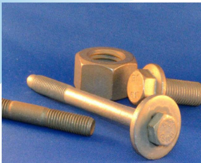
Mechanical plating can be used to apply zinc, tin or aluminium coatings, either singly or in combination.
